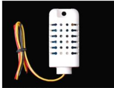
AM2302/DHT22 with big case and wires
