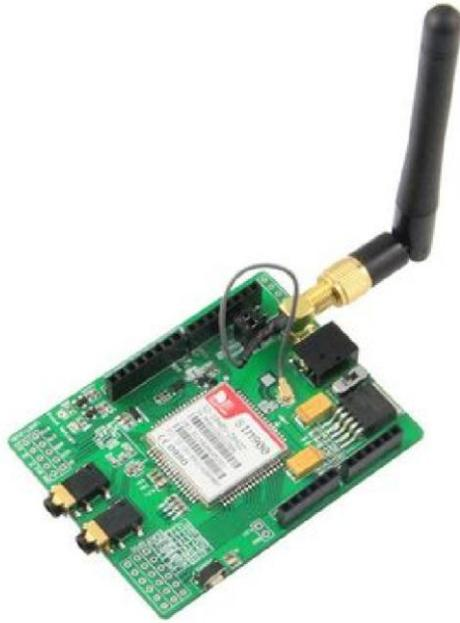
The GPRS Shield is based on SIM900 module from SIMCOM and compatible with Arduino and its clones. The GPRS Shield provides you a way to communicate using the GSM cell phone network. The shield allows you to achieve SMS, MMS, and GPRS and Audio via UART by sending AT commands (GSM 07.07 ,07.05 and SIMCOM enhanced AT Commands). The shield also has the 12 GPIOs, 2 PWMs and an ADC of the SIM900 module(They are all 2V8 logic) present onboard
