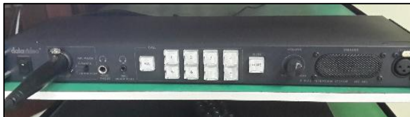
Fig. 4. 9: 8 Way Intercom System ITC-100
