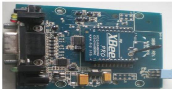
**Figura 6.4:** Radio modem XBEE PRO.
