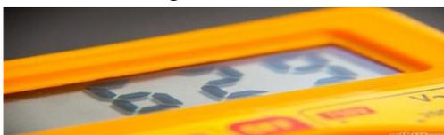
**4) Move the red probe to the collector.** The display should give the same reading as when you touched the probe to the emitter.
