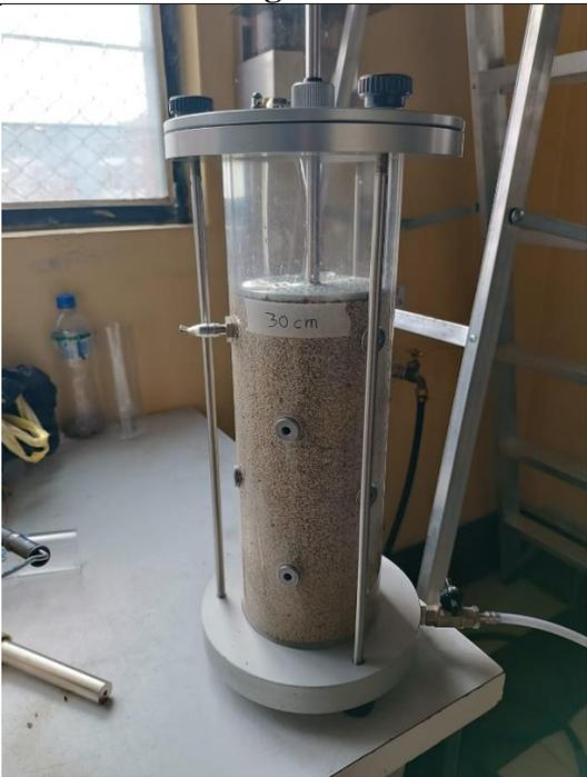
A photograph of the permeameter assembly on a table. The chamber is filled with granular material. A white label with the text "30 cm" is attached to the side of the chamber. The device is connected to a water supply line. |
