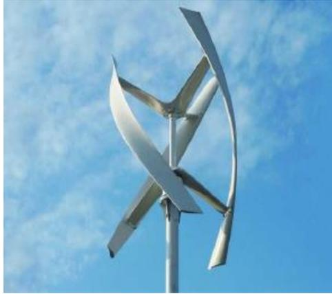
**Figura 1.7:** Rotor Darrieus helicoidal [11].
