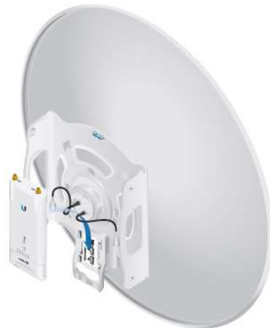
Mounting a Rocket on the RD-5G30-LW
