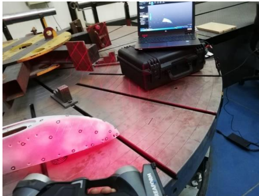
Figura 19.- Scanner HandySCAN 3D.
