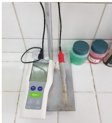
Figura 4. pH-metro METTLER TOLEDO Five GO
