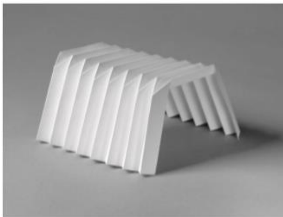
5.2_2 The use of two lines of v-folds creates a span with a flat "roof". Note how the two lines are mirror images of each other.
