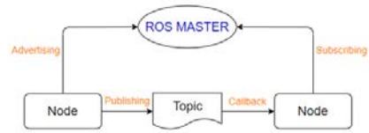
Fig. 3. Component system of a ROS model
