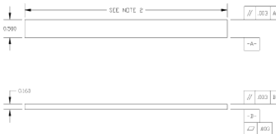
FIG. 5 Standard Flexural Test Specimen Drawing (Inch-Pound)
