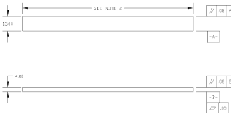
Note 1—Drawing interpretation per ANSI Y14.5-1999 and ANSI B46.1-1995. Note 2—See 8.2 and 11.3 of this test standard for the required values of span and overall length. FIG. 4 Standard Flexural Test Specimen Drawing (SI)
