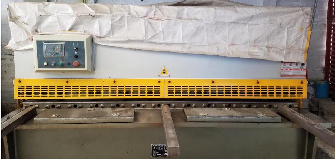
**Figura 18.-** Cortado industrial (Hydraulic Shearing Machine)
