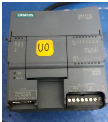
Fig. 6.13. PLC s71200, CPU 1212C, ACDC Relay
