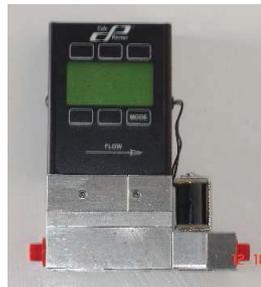
**Figura 2.11** Water Flow Controller LC-500CCM-D
