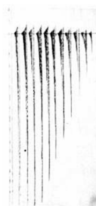
FIG. 12 Sample Drum Record of Impact Bending Test
