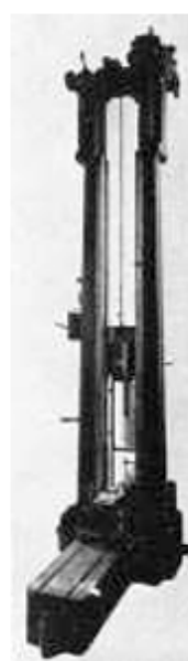
FIG. 11 Hatt-Turner Impact Machine, Illustrating Method of Conducting Impact Bending Test
