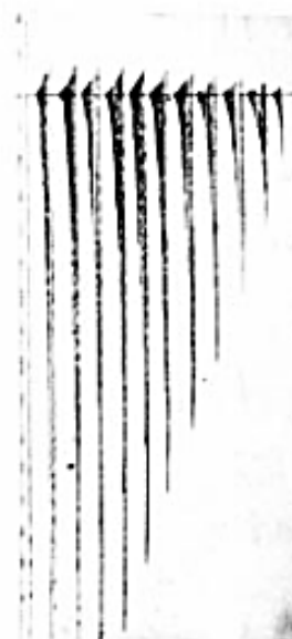
FIG. 12 Sample Drum Record of Impact Bending Test
