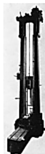
FIG. 11 Hatt-Turner Impact Machine, Illustrating Method of Conducting Impact Bending Test
