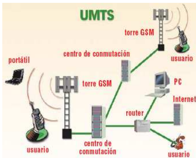
Figura 2.26 Diagrama de Red UMTS. Obtenida de: http://lh6.ggpht.com/_t7heG8GISSo/TKkvFCSUK4I/AAAAAAAAADzo/OZ_wltNHtjg/umts.png
