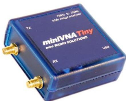
The miniVNA Tiny, is a handheld pc based Vector Network Analyzer that makes available a multitude of features and capabilities which are perfect for checking antennas and RF circuits for hams and commercial users **from HF to SHF.**
