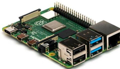
**Figura 25:** Servidor Raspberry Pi 4. [59]
