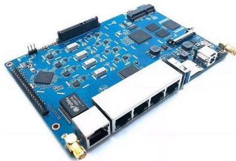
**Figura 24:** Servidor Banana pi r64. [58]
