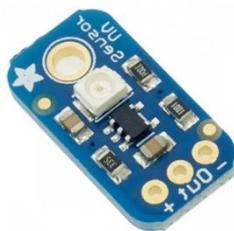
**Figura 11:** sensor ultravioleta GUVA-S12SD [34].
