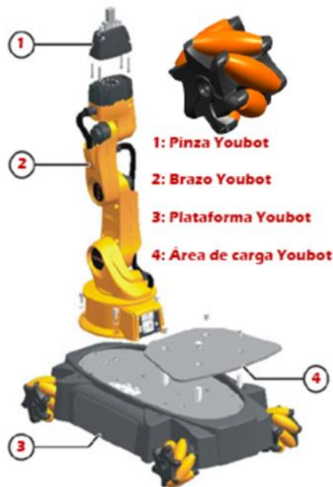
Figura 8: Hardware Youbot Fuente: Investigador (Photoshop)
