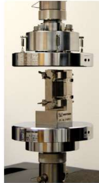
▲ Anti-buckling fixture with base support end loaded between compression platens. The upper compression platen has a lockable spherical seat
