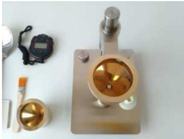
Figura 2-1 ISO 4490 Metallic powders flow rate Hall flow meter. Fuente: [1]
