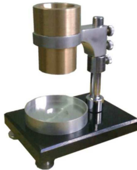
Figura 2-4 ISO13517 Metallic powder Gustavsson flow meter product. Fuente: [4]
