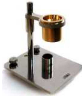
Figura 2-3 ASTM B964 Metal Powders Carney Funnel Flowrate Meter. Fuente: [3]
