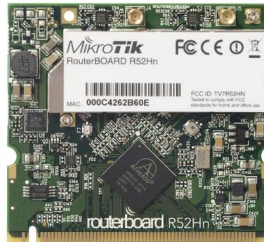
**Figura 6.45.** Router Board RB52Hn
