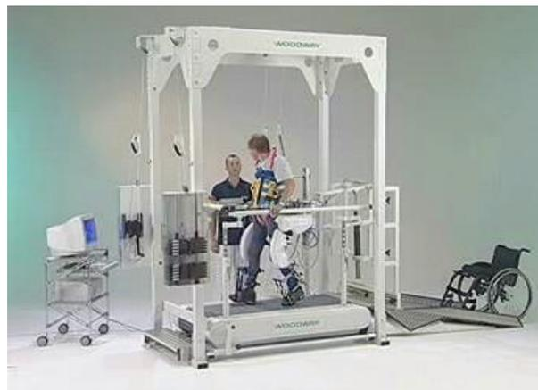
Figura 5: Órtesis Lokomat
