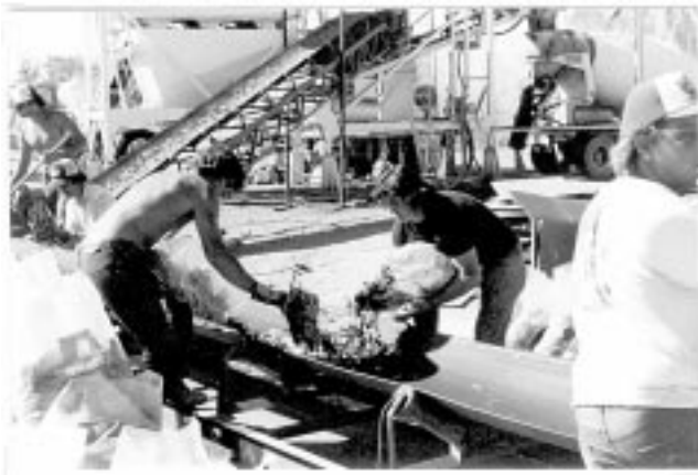
Fig. 2.8—Adding steel fibers via conveyor onto charging conveyor in a batch plant
