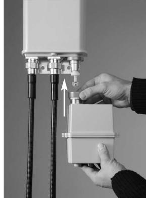
Push the attachment nut of the RCU down towards the housing.
