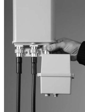
Tighten the RCU attachment nut using a torque-wrench; wrench width = 41 mm, min. torque = 15 Nm, max. torque = 18 Nm.
