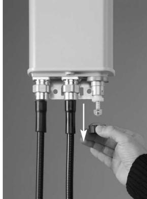
Completely remove the black adjustment wheel by simply pulling it downwards.
