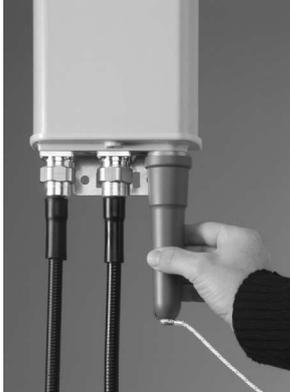
Remove the protective cap completely from the antenna.
