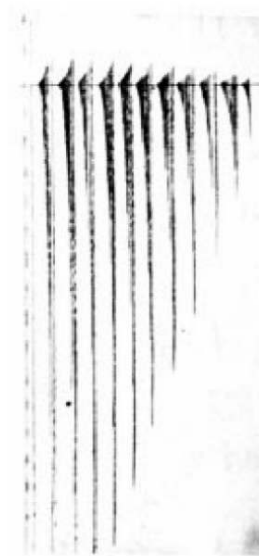
FIG. 12 Sample Drum Record of Impact Bending Test
