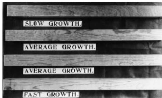
FIG. 2 Tangential Surfaces of Bending Specimens of Different Rates of Growth of Jeffrey Pine 2 by 2-in. (50 by 50 by 760-mm) Specimens
