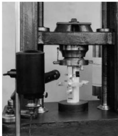
FIG. 9 Compression-Parallel-to-Grain Test Assembly Showing Method of Measuring Deformations by Means of Roller-Type Compressometer
