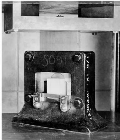
FIG. 22 Shear-Parallel-to-Grain Test Assembly Showing Method of Load Application Through Adjustable Seat to Provide Uniform Lateral Distribution of Load
