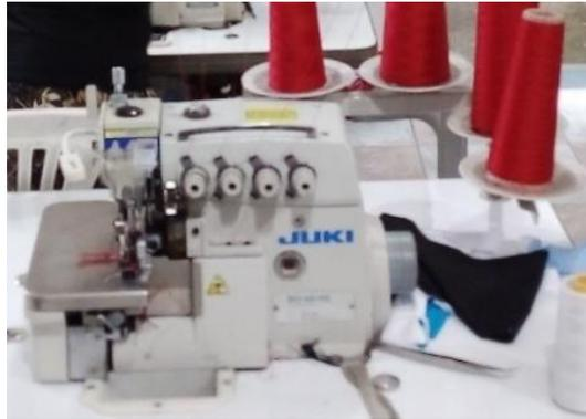
**Figura 17:** Máquina overlock.
