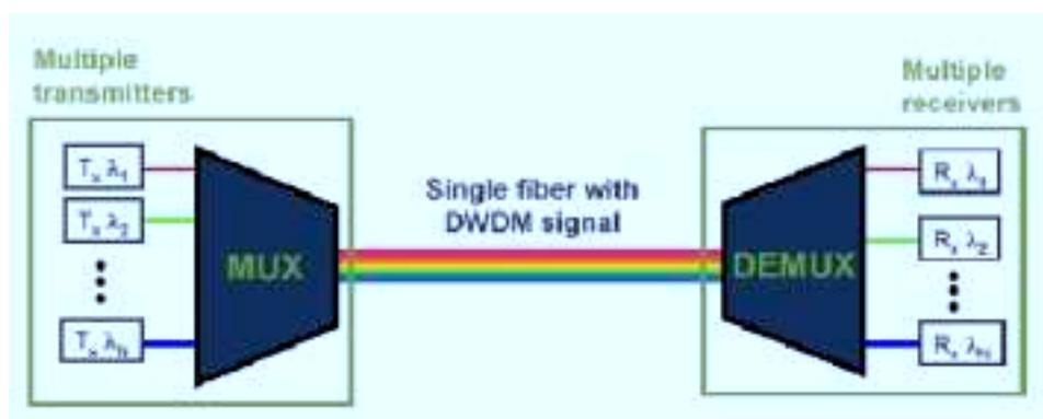
**Figura3.1.DWDM (Dense Wavelength Wavelength)**
