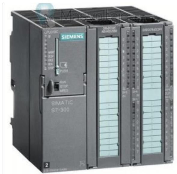
**Figura 1.3.6:** PLC's Siemens.
