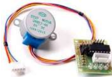
Figura. 2-48 Motor unipolar 28BYJ-48 con el Driver ULN2003 [47]
