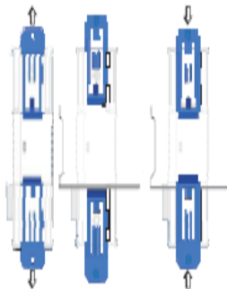
FIG-1 Pull up the sliders provided with the unit towards outward direction. FIG-2 Rest the unit on the DIN rail plate FIG-3 Pull down the slider again so that unit can fix up with the DIN rail plate.
