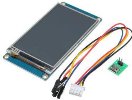
Figura 4.5 Pantalla nextion 3.5 pulgadas [43].
