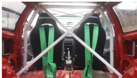
Figura 7 Arco principal Roll bar artesanal
