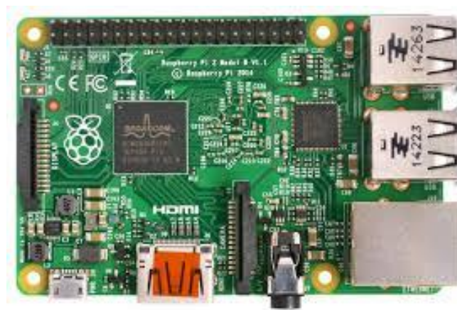
Figura 14. Raspberry 1 Model B+. [26]
