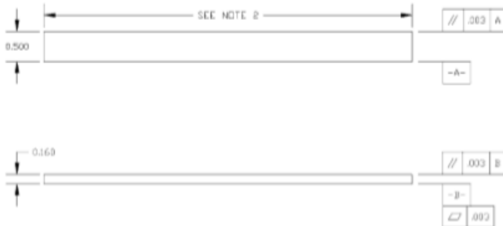
Nom 1—Drawing interpretation per ANSI Y14.5-1999 and ANSI B46.1-1995. Nom 2—See 8.2 and 11.3 of this test standard for the required values of span and overall length. FIG. 5 Standard Flexural Test Specimen Drawing (Inch-Pound)
