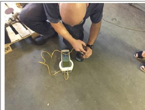
Pic.43: Calibrating hardness tester device with pattern
