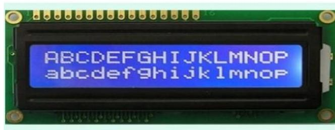
**Fig.39:** LCD 16 x 2. [35]
