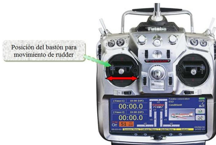
**Figura 4. 35: Bastón Rudder**
