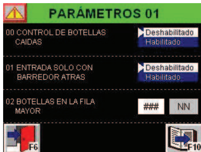
Fig.11._ Pantalla Parámetros 01 terminal HMI Panel View Plus 600 (Stacker)
