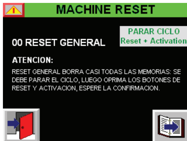
Fig. 6._ Pantalla Reset General terminal HMI Panel View Plus 600 (Stacker)
