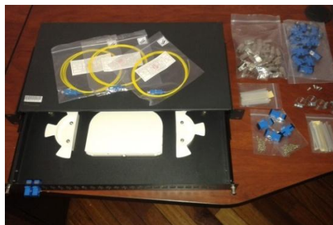
Figura 6.27: ODF (Optical Distribution Frame)
