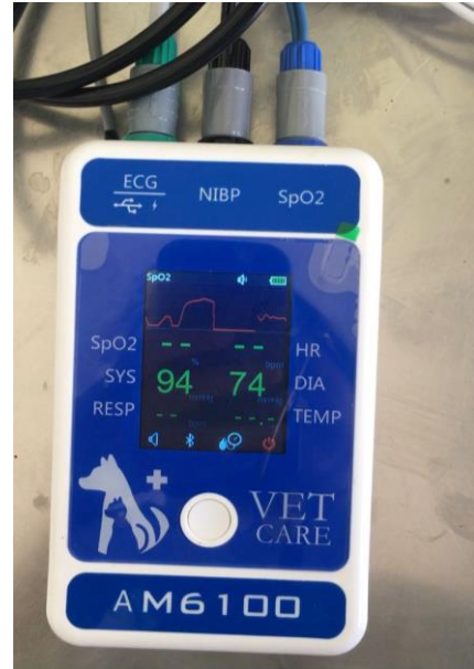
Monitor AM6100: SpO 2 sensor (Cable azul) y NIBP Hose (Cable negro)
