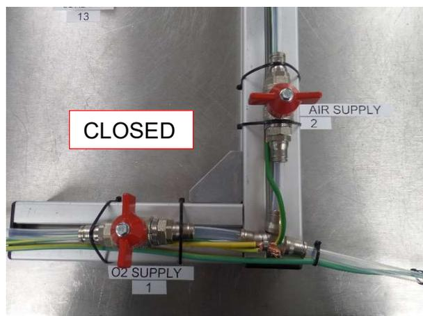
Figure 9: Oxygen [1] and Air [2] supplies are CLOSED
