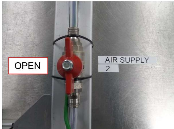
Figure 34: Air supply valve OPEN
