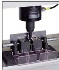
• **PC card insertion and removal test jig**
