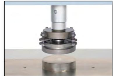
Spherical seat type compression plates
