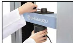
Load cell attach/release
