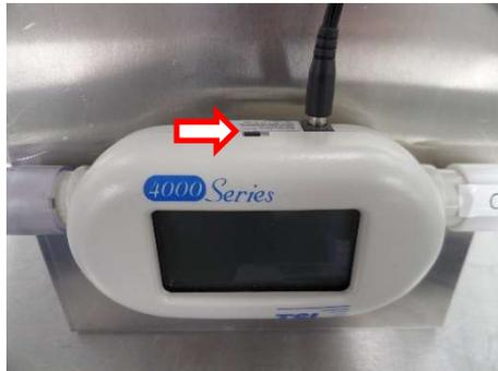
Figure 5: ON/OFF Switch
