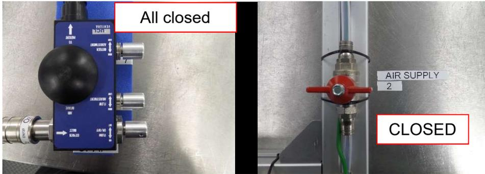
Figure 38: On/Off valve CLOSED
