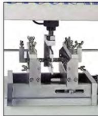
• **Long-span 4-point bending test device for wooden specimens**
