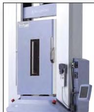
• **Device for torsion test in thermostatic chamber**
