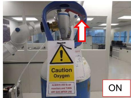
Figure 11: Handle lifted, bottle ON
