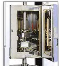
• **Bellows-type long stroke thermostatic chamber**
