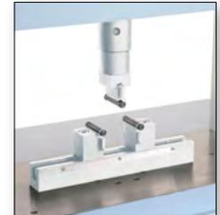
3-point bending test of plastic specimen
