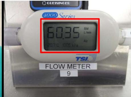
Figure 29: Flow meter shows 60 L/min
