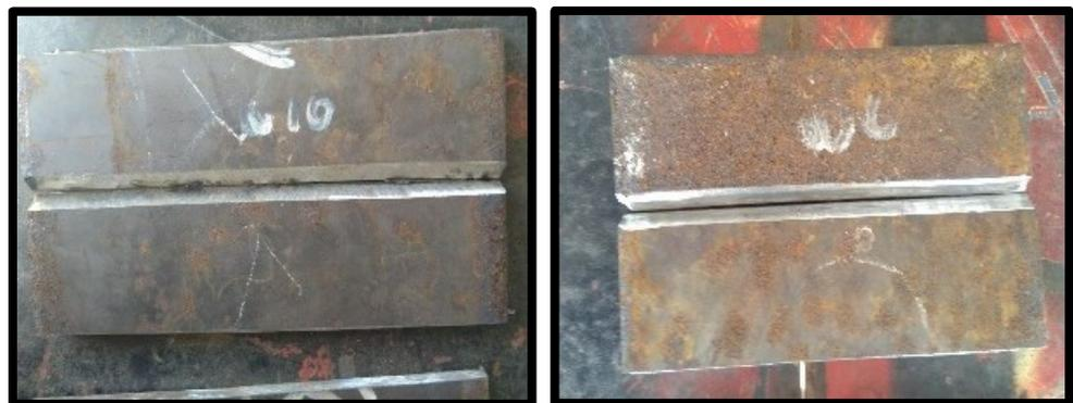
**Figura 2.3. Placas preparadas de 190x100x8 mm y 150x100x8 mm**
