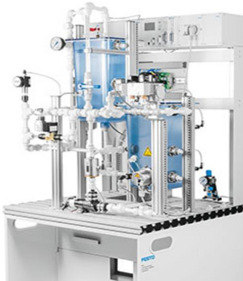
Figura 31: Célula analógica FESTO MPS PA® Compact Workstation.
