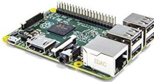
Fig. 2.25: Raspberry Pi 2 modelo B+, [40]
