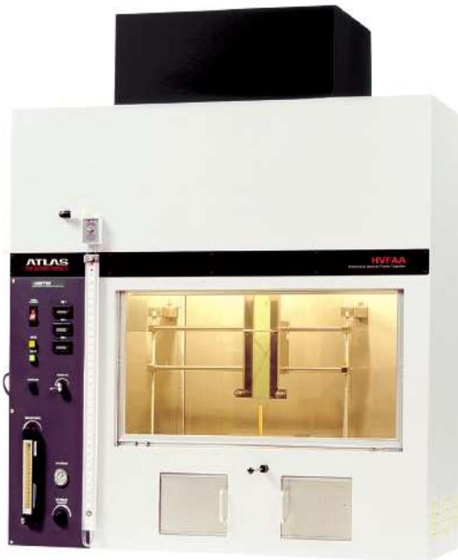
Atlas' HVFAA Horizontal Vertical Flame Chamber accurately determines the flammability of cabin compartment materials and electric wire. The chamber is designed to perform Bunsen burner tests in accordance with FAA's *Aircraft Material Fire Test Handbook* DOT/ FAA/AR-00/12, chapters 1.0 - 4.0 (FAR 25.853, 25.855, 25.1359).
